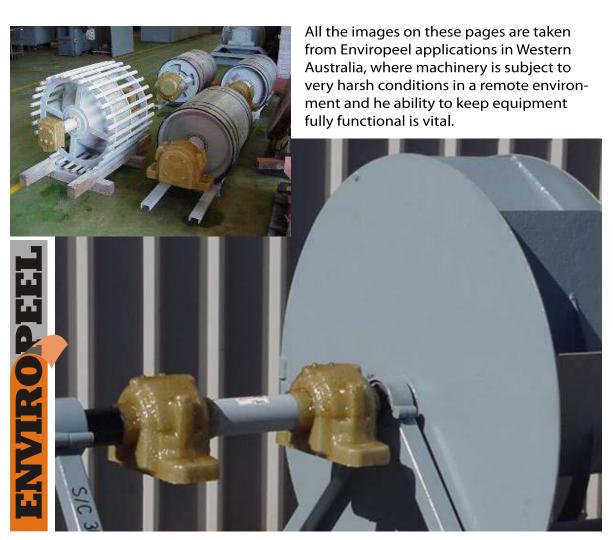
With a vast range of rotating equipment of all sizes, cooling fans, drums and pumps, BHP use Enviropeel to protect the entire bearing housing because it does not need to be removed for use. But, if removal is required, it only takes a few seconds, as the picture on the right shows with the bearing emerging as good as new!
