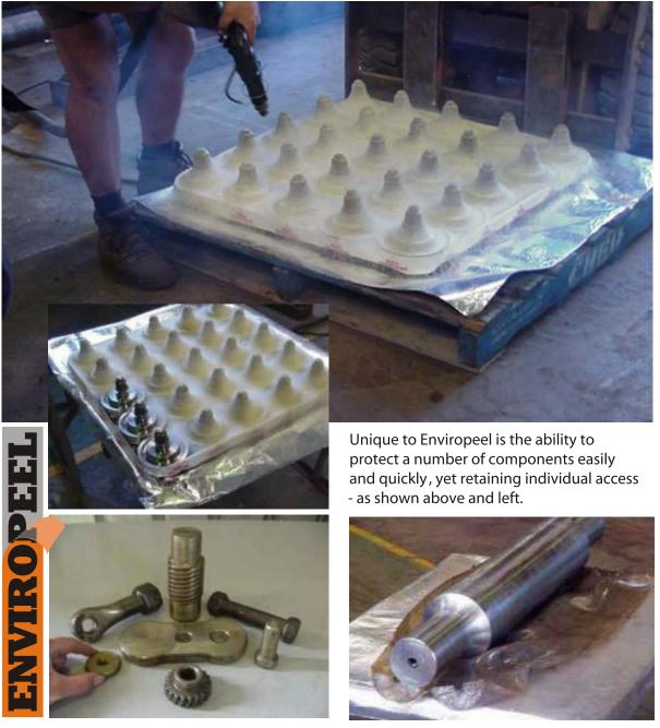
Enviropeel is suitable for the protection of components, large or small, with the ability to vary the application type to suit the requirement - short or long term, transit and abrasion as well as anti- corrosion. All without waste or any threat to the environment.
